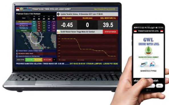
Figure 4.2: Groundwater level (GWL) monitoring interface developed under the BRG–JICA cooperation. Screenshot from the BRGM Project Final Report showing a laptop and a mobile-phone application used to visualize peatland groundwater levels, rainfall, soil moisture, and short-term weather forecasts, enabling Indonesian and Japanese partners to track fire risk in near-real time and support decisions on canal blocking and rewetting. Source: https://openjicareport.jica.go.jp/pdf/12320909_01.pdf
